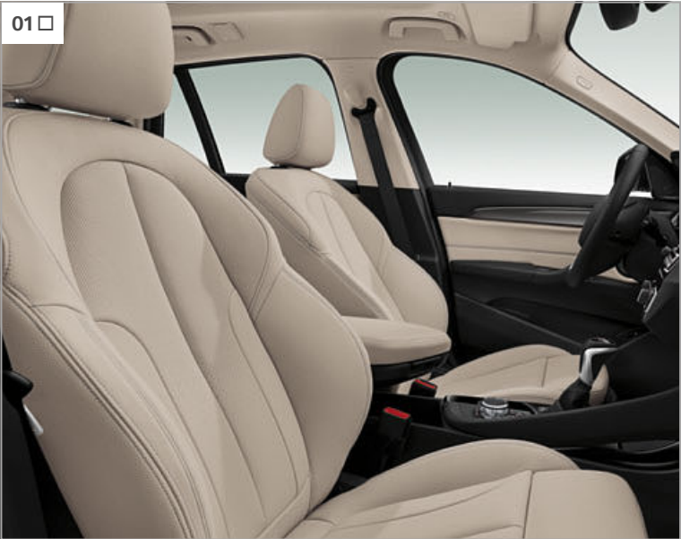
[ 01 ] The optional sport seats, shown here in the optional leather 'Dakota' with Oyster perforations and Grey accents, give particularly good lateral support thanks to the larger bolsters on the seat surfaces and backrests, and can be adjusted in various ways.
