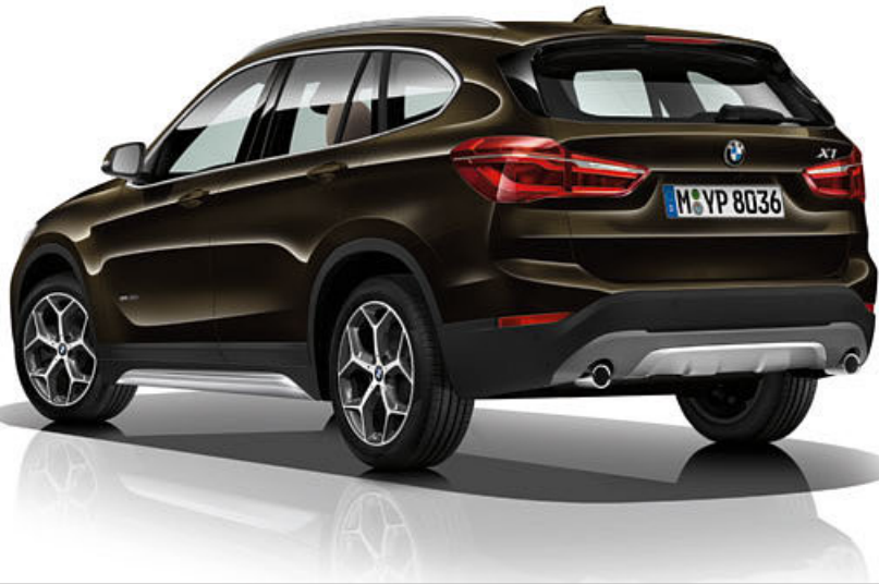
[ 05 ] 18" light alloy wheels Y-spoke style 569, tyre size 7.5J x 18 with 225/50 R18 tyres.
