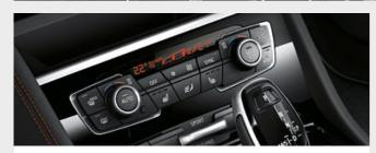
☐ The Automatic air conditioning with two-zone control<sup>2</sup> and automatic temperature control features separate controls for the driver and front passenger. It also includes Automatic Air Recirculation (AAR), a Microactivated carbon particulate filter, a fogging and solar sensor, as well as rear air vents.
