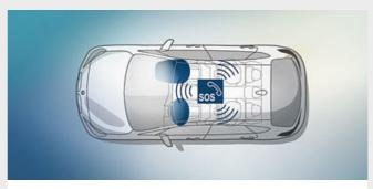
☐ The Intelligent Emergency Call automatically establishes a connection with the nearest rescue coordination centre through the BMW call centre whenever needed - without the use of a mobile phone. It transmits information regarding the vehicle's current location and the severity of the accident. The Intelligent Emergency Call can also be triggered manually in case other road users require help, for example.
