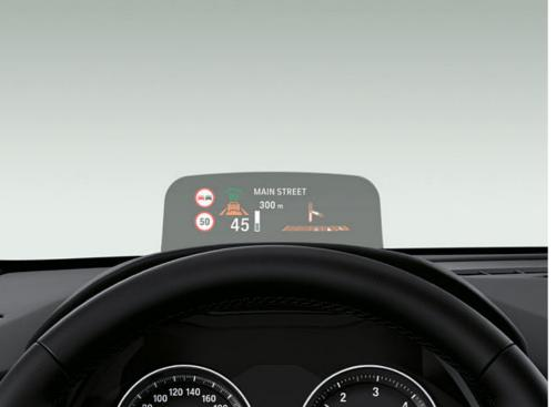
☐ The full-colour BMW Head-Up Display<sup>1,8</sup> projects all relevant driving information onto a panel in the driver's field of vision, which means they can remain focused on the road. Current speed, directions from the navigation system, Speed Limit Info incl. no-overtaking indicator and telephone and entertainment lists, among other things are displayed.
