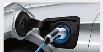
The port for external charging of the high-voltage battery is located behind a flap on the vehicle's front side panel on the left. The charging port is protected from the elements by a special seal. The LED light ring around the port indicates the vehicle's current charge status.
