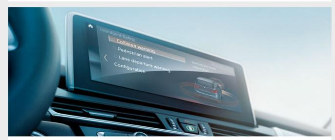
The safety package **Driving Assistant**<sup>1,2,5</sup> includes camera-based assistance systems, such as Lane Departure Warning, Approach control warning, High-beam assistant and Speed Limit Info. The Approach control warning and Person warning with light city braking function warns of collisions at speeds between 10 and 60 km/h, while the Lane Departure Warning causes the steering wheel to vibrate as a warning when the lane is unintentionally changed at 70 km/h or over.
