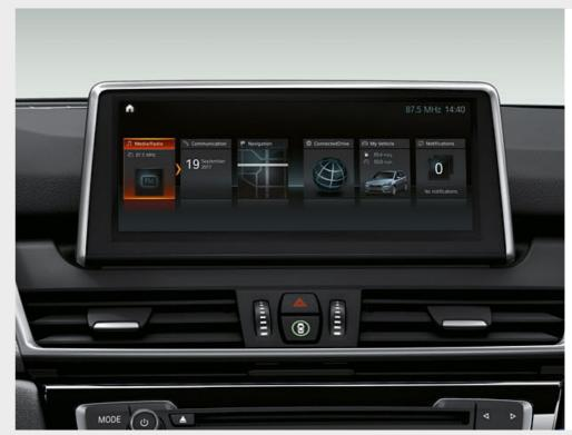
☐ Navigation Plus³ features a BMW Head-Up Display<sup>1</sup>, an iDrive Touch Controller, a built-in 8.8" touch display and an instrument cluster with high-resolution 5.7" TFT display. The system is operated intuitively using either the iDrive Touch Controller, the direct menu control buttons and six or eight functional bookmarks, voice control or the touchscreen with interactive tiles.
