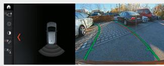
☐ The Rear view camera® enables improved orientation when reversing at speeds below 15 km/h, for example when parking. It shows the area behind the car on the Control Display. Interactive track lines for measuring distance and turning circles assist you when manoeuvring. Obstacles are marked in colour.
