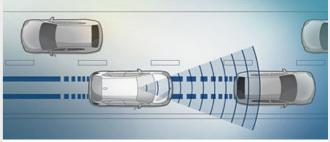
☐ Approach control warning with light city braking function<sup>1, 3</sup> warns of potentially critical situations to help prevent accidents. If there is a risk of collision with a vehicle moving or standing ahead, it provides a two-stage warning and, if necessary, pre-conditions the brakes for increased responsiveness. In case of an emergency, the system initiates braking, ensuring that the collision speed is significantly reduced.
