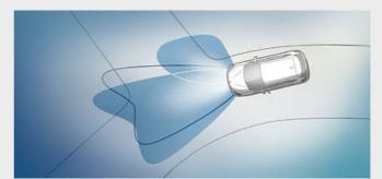
☐ The **Adaptive LED headlights** include low-beam and highbeam headlights and turn indicators with full LED technology. The equipment also features BMW Selective Beam, cornering lights, daytime running lights and Adaptive headlights with variable light control for excellent illumination of the road ahead and better visibility in the dark.
