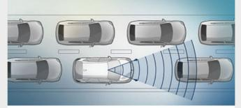
☐ **Traffic jam assistant**<sup>4,5</sup> relieves you in monotonous traffic situations on the motorway: At speeds of up to 60 km/h, the system lets the car simply "glide along" with the other cars in dense traffic, making traffic jams less stressful. It automatically maintains the distance from the vehicle ahead and regulates the car's speed down to a standstill - as well as providing steering support.
