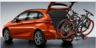
O The foldable Compact rear bike rack is light but sturdy and can carry up to 60 kg. It can be quickly and securely mounted on the tow ball and transport up to two bicycles or e-bikes. When folded up, it can be stored in the luggage compartment tray, safe from spray and protected in the event of a collision.
