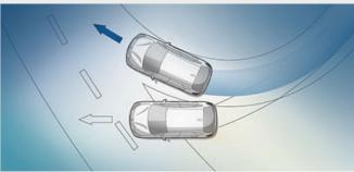
■ Dynamic Stability Control (DSC) continuously assesses the vehicle's movements using various sensors and stabilises the car with engine and braking regulation when unstable driving conditions are detected. Auxiliary functions include braking readiness, brake drying by the braking system in wet conditions and the Hill-Start assistant.
