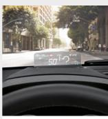
O The Head-Up Screen puts vehicle information and, in combination with a smartphone interface, navigation information into the driver's line of sight.
