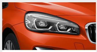
☐ The Adaptive LED headlights include low-beam and high-beam headlights and turn indicators with full LED technology. The equipment also features BMW Selective Beam, cornering lights, daytime running lights and Adaptive headlights with variable light control for excellent illumination of the road ahead and better visibility in the dark.
