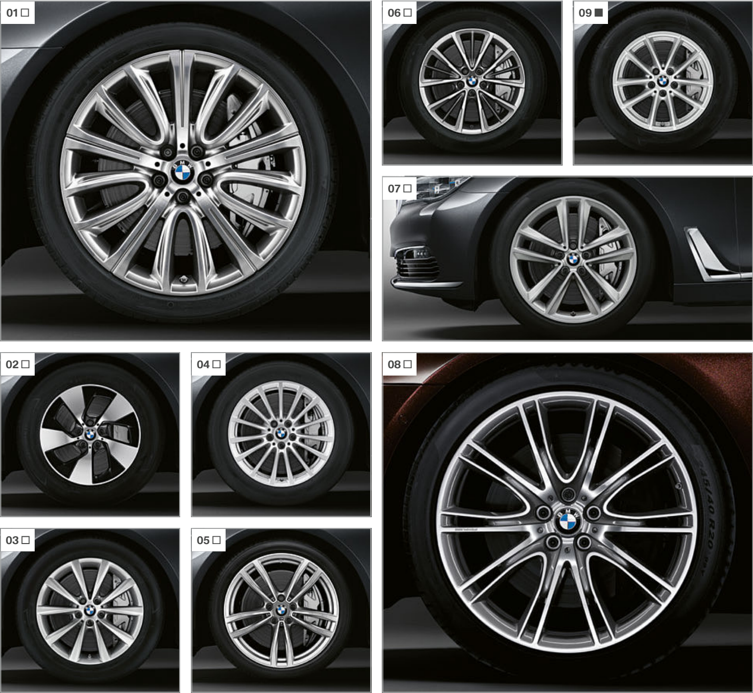
[ 01 ] 20" light alloy wheels V-spoke style 628 1 , Bicolour, with mixed tyres and runflat properties. Front: 8.5 J x 20 with 245/40 R 20 tyres. Rear: 10 J x 20 with 275/35 R 20 tyres. [ 02 ] 17" light alloy wheels Turbine styling 645 1,2 , Bicolour, BMW EfficientDynamics. Wheels: 7.5 J x 17. Tyres: 225/60 R 17. The design helps to reduce fuel consumption and CO 2 emissions. [ 03 ] 18" light alloy wheels V-spoke style 642 1 . Wheels: 8 J x 18. Tyres: 245/50 R 18.
