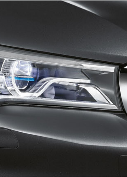
[ 10 ] When the high beams are on, BMW Laserlight 3 doubles maximum illumination range, reaching up to 600 metres. Includes Adaptive headlights and BMW Selective Beam (anti-dazzle High-beam assistant).
