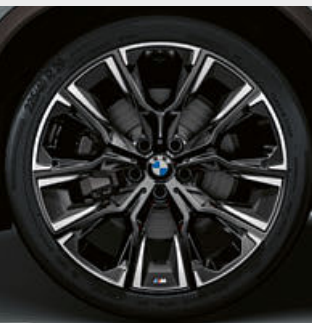
□ 20" M aerodynamic wheels 920 M Bicolour Midnight Grey with run-flat tyres, gloss-lathed, wheel size 8J x 20 with 225/40 R20 tyres. 4
