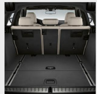
□ The luggage-compartment package\* enhances the functionality of the luggage compartment, e.g. backrest tilt adjustment including cargo position and lashing rails.
