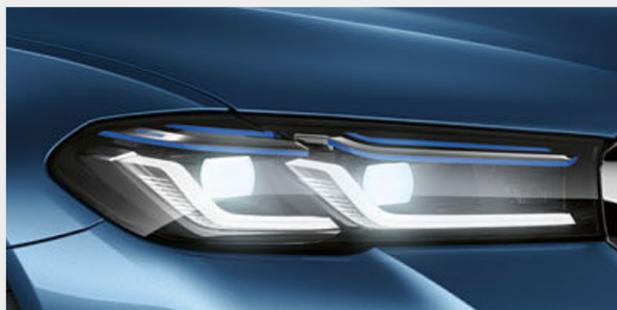
□ In laser high-beam mode, BMW Laserlight\* illuminates a range of up to 650 m, nearly twice as far as that of conventional headlights. Better visibility in the dark significantly increases safety. Blue accents and the lettering "BMW Laser" in the headlight also underline the technological standards and the sportiness of the vehicle.
