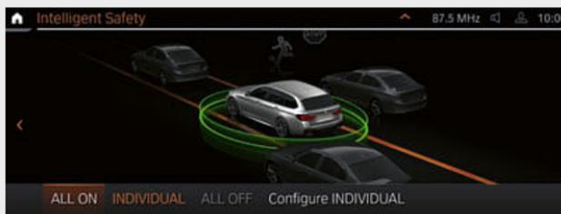
□ Driving Assistant Professional<sup>3</sup>\* offers optimum comfort and safety during critical or monotonous traffic situations. Apart from the contents of the Driving Assistant, it also includes Steering and Lane Control Assistant with extended functions, Emergency Stop Assistant and Lane Keeping Assistant with active side collision protection.
