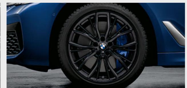
○ The high-quality 19" M Performance forged wheel Double-spoke style 786 M is designed in Jet Black matt with the colour M logo and milled M Performance lettering. TPMS winter complete rear wheel with run-flat tyre, wheel size 9J x 19, tyre size 275/35 R19 100V XL RSC.
