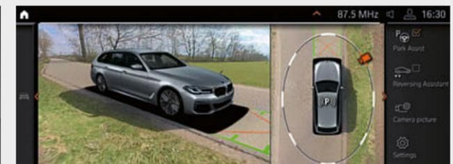
□ The equipment package Parking Assistant Plus\* makes parking and manoeuvring the vehicle easier. It features Surround View including Top View, Remote 3D View, PDC as well as a lateral parking aid, the Active PDC emergency braking function and the Parking Assistant with linear guidance<sup>5</sup> that provides fully automatic parking both parallel and perpendicular to the road.
