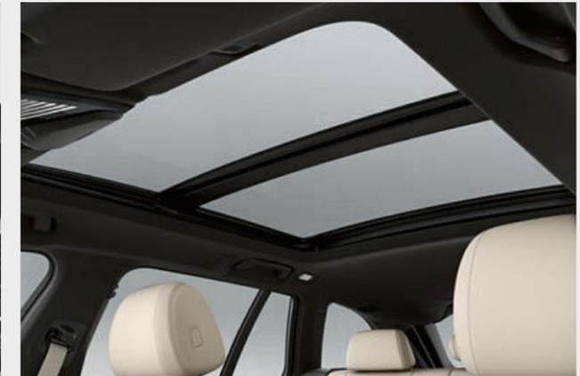
□ When open, the Panorama glass roof provides a great deal of fresh air. Closed, it creates a bright, light-flooded atmosphere in the interior. It opens and closes completely automatically at the push of a button or with the car key, and is equipped with slide and lift functions, roller sunblind and wind deflector.
