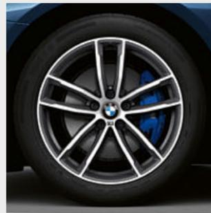
□ 18" M light alloy wheels Double-spoke style 662 M Orbit Grey with mixed tyres, gloss-lathed, wheel size front 8J x 18 with 245/45 R18 tyres, wheel size rear 9J x 18 with 275/40 R18 tyres.<sup>2</sup>
