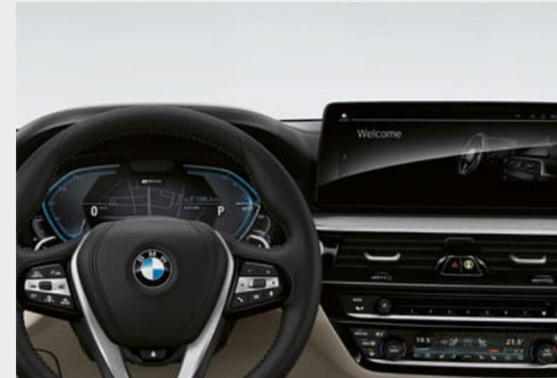
□ The BMW Live Cockpit Professional\* with navigation function includes two high-quality displays consisting of a high-resolution 12.3" Control Display that can be operated by touch and a fully digital 12.3" instrument display. The BMW Operating System 7 can also be operated via the iDrive Touch Controller.
