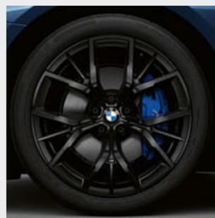
□ 19" M light alloy wheels Y-spoke style 845 M Jet Black with mixed tyres, wheel size front 8J x 19 with 245/40 R19 tyres, wheel size rear 9J x 19 with 275/35 R19 tyres.<sup>2</sup>
